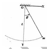
A rigid body of mass m is suspended from point O using an inextensible string of length L. When it is displaced through an angle  $\theta$ , what is the change in the potential energy of the mass? (Refer adjacent figure.)
