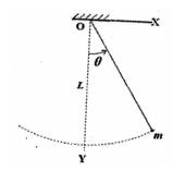
A rigid body of mass m is suspended from point O using an inextensible string of length L. When it is displaced through an angle  $\theta$ , what is the change in the potential energy of the mass? (Refer adjacent figure.)
