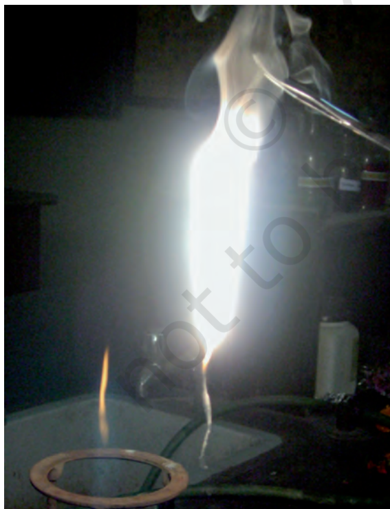
Fig. 6.3 Magnesium ribbon burning
