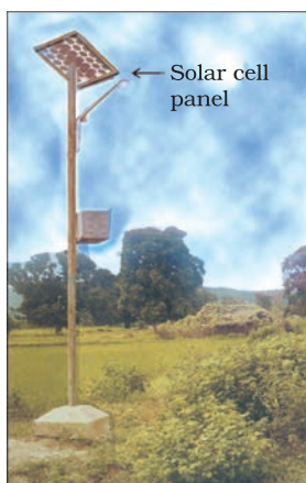
Figure 14.7 A solar cell panel
