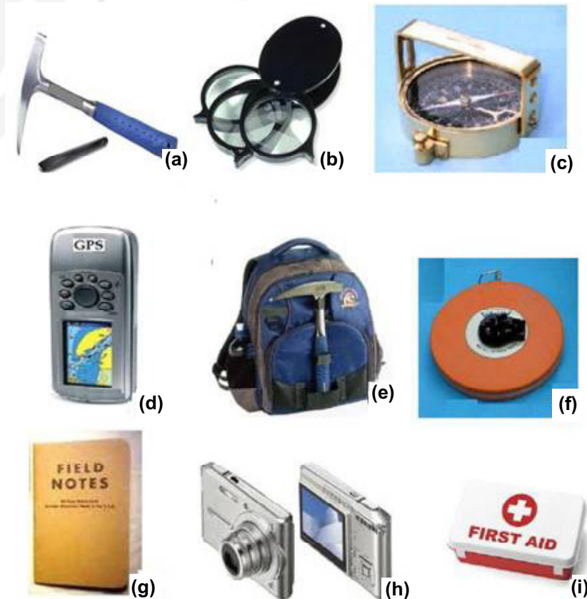
Fig. 13.4: Field equipment (a) hammer and chisel, (b) hand lens, (c) clinometer, (d) GPS, (e) haversack, (f) measuring tape, (g) field notebook, (h) digital camera, and (i) first aid box
