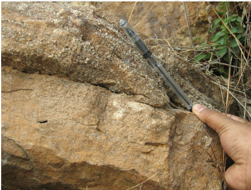
Fig. 13.8: Medium grained sandstone overlain by very coarse grained sandstone. Quartz mineral can be identified in very coarse grained sandstone with naked eye.
