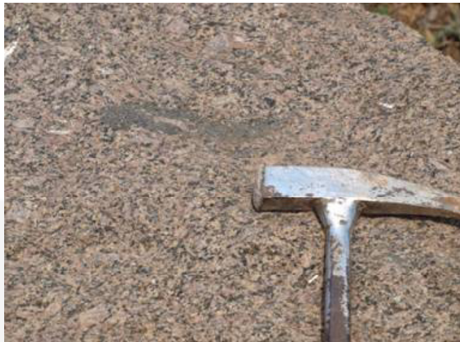
Fig. 13.6: (a) Interlocking texture observed in igneous rocks when examined rock under hand lens, and (b) Granite in handspecimen
