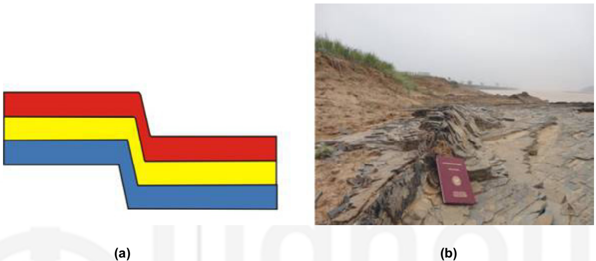
Fig. 10.22: Monocline: a) Sketch; and b) Field photograph.
