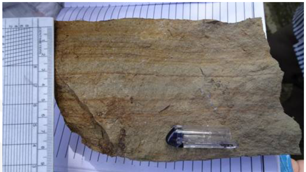
Fig. 9.1: a) Sketch showing stratification with numerous beds, bedding planes and laminations; and b) Field photograph showing planar laminations, parallel to cap of pen. (Photo credit: Ganga Prasad Bhartiya)
