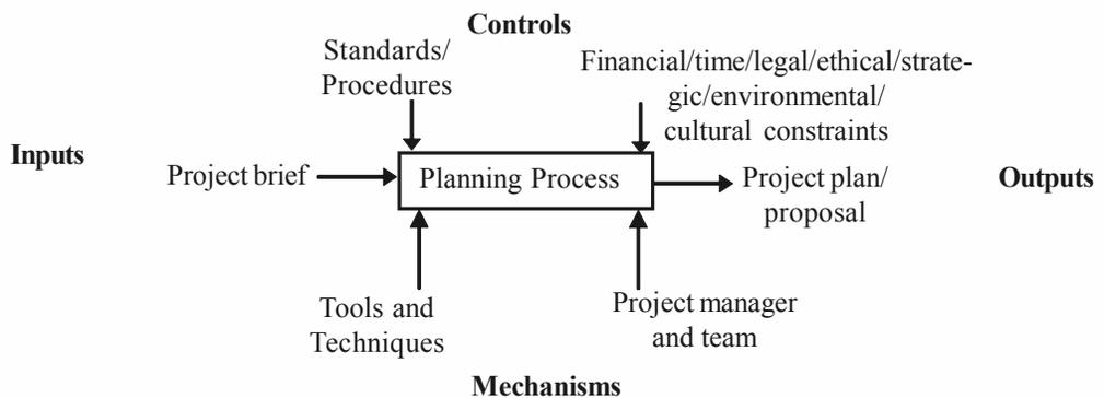
Fig. 4.7: Activity model using ICOMs
