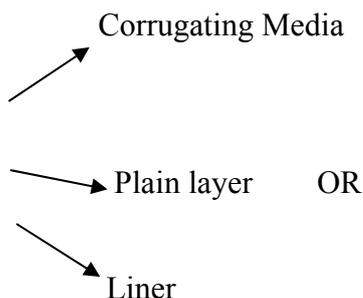
Subsequently, the 2 ply corrugation roll could be converted into 3 ply corrugated fibre board by pasting another Kraft liner or facing material. In the same manner, corrugated fibre board could be made either of 3 ply or 5 ply or 7 ply by means of pasting the corrugation roll and facing material. This could be illustrated with the following diagram.
