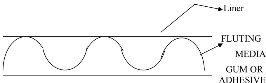
**3 Ply or Single Wall Corrugated Fibre Board.**
