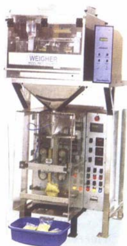
Figure 14.3: A form-fill-seal machine
