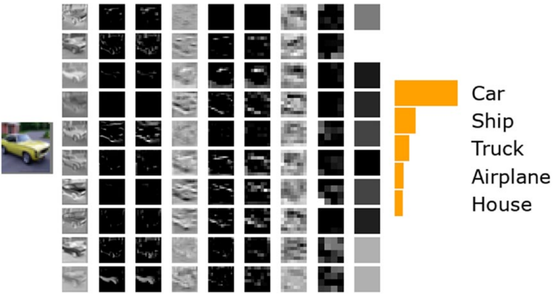
Figure 5-14. How the filters extract features
