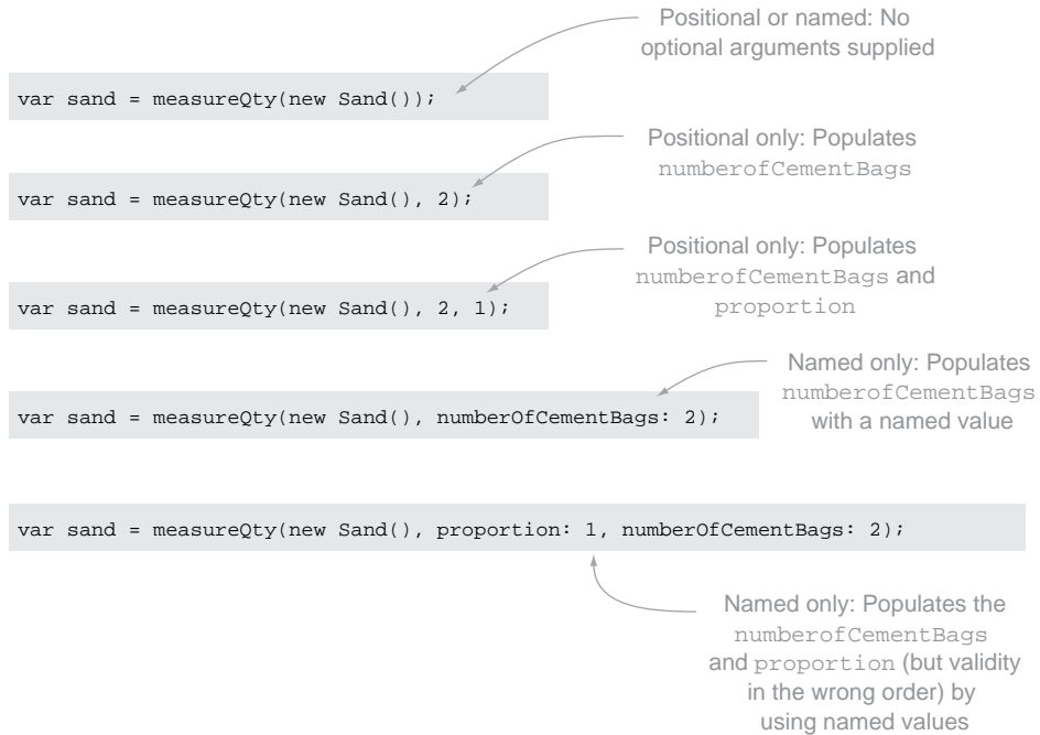
Figure 4.4 The different ways that calling code can supply values for optional positional and named function parameters
