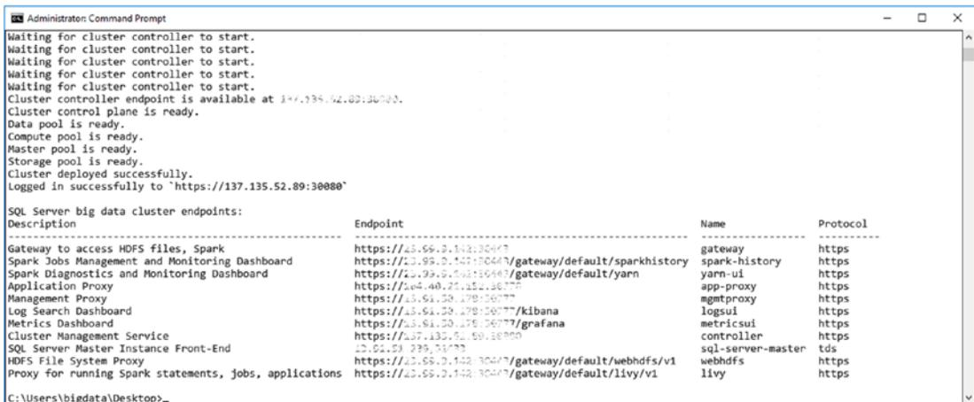
Figure 3-25. Final output of Python deployment script including IP addresses
