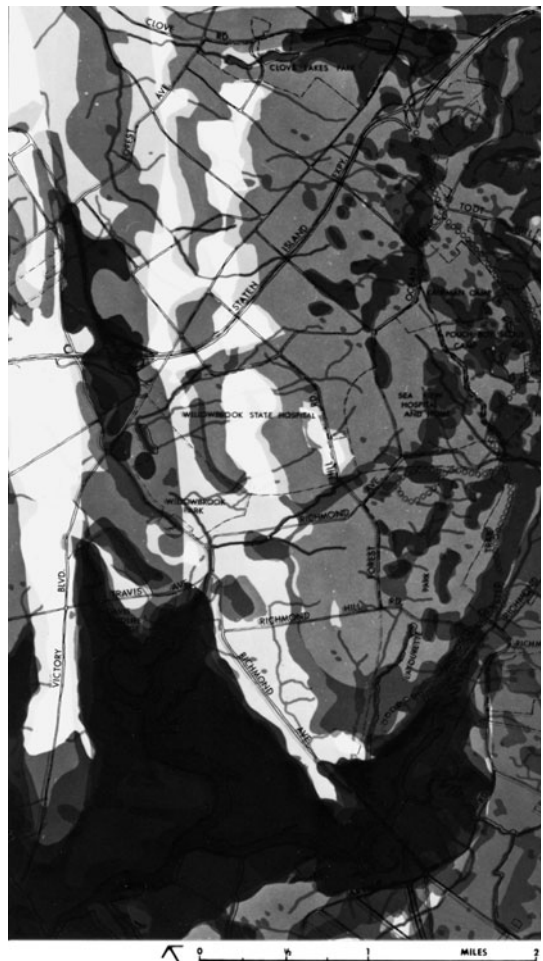
Figure 14.1 Acetate overlay to determine environmental sensitivity. Example of Ian McHarg’s use of manual acetate overlay operations to illustrate increased sensitivity as a number of categories of physical parameters overlap. This map shows the overlapping of slope, surface drainage, bedrock foundation, soil foundation, and susceptibility to erosion for the Richmond Parkway study area in New Jersey. Source: Ian McHarg, Design with Nature , John Wiley & Sons, New York, © 1995. Reprinted with permission.
