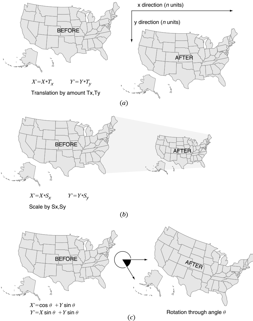
Figure 6.6 Translation, scale change, and rotation. The three basic graphic transformations necessary to make the projection transformations: (a) translation, or object movement within the coordinate space; (b) scale change, to adjust the object size; and (c) rotation, to reorient the object within the coordinate space.
