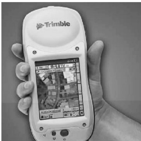
Figure 6.10 Integrated iPAQ and GPS technology illustrated by this Trimble® GeoXT GPS unit with built-in Hewlett Packard iPAQ® and ESRI ArcPad software.
