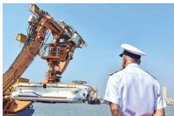
Help at hand: The deep-submergence rescue vehicle can go up to a depth of 650 metres. • FILE PHOTO
