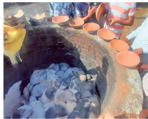
Heat loss: About 25% of the clay griddles break during baking in the kilns. • SPECIAL ARRANGEMENT
